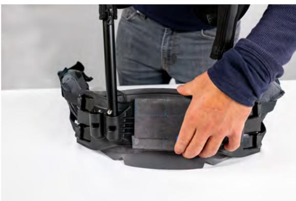
4. Lift Ekso EVO off your shoulders and disassemble arms from the hip belt by pressing the silver buttons on the bottom of the torso tubes. Place all components back into the Ekso carrying bag.
