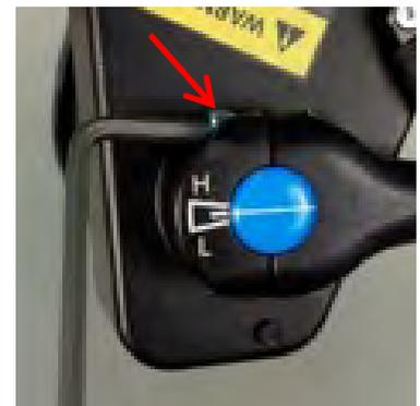
**Figure 17: Loosening End Link Screw**
